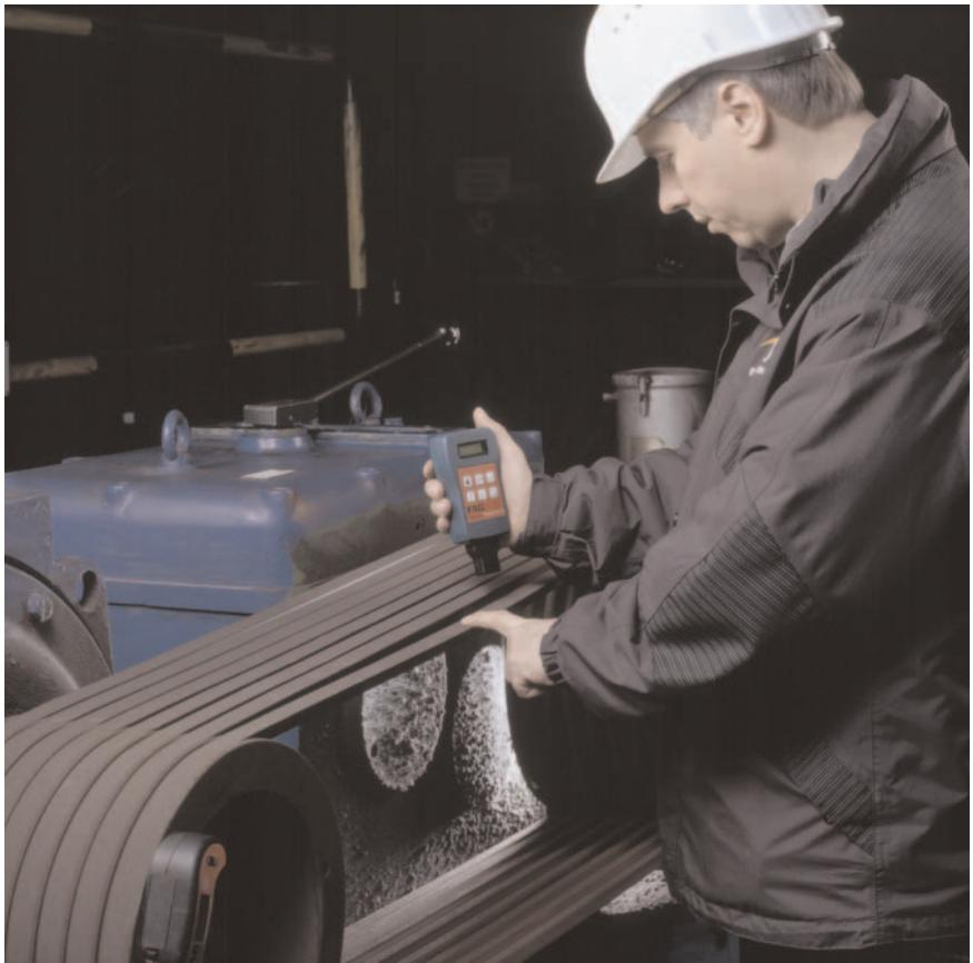
Measurement using cableless measurement probe
