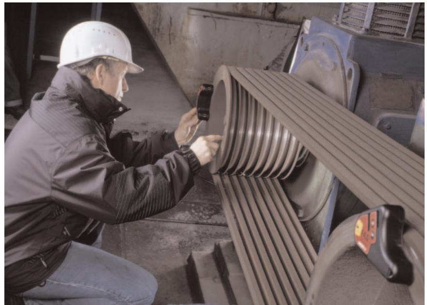
Alignment of belt pulleys
