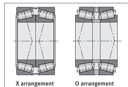
The same grippers are used in reverse for an O arrangement of the tapered roller bearings.
