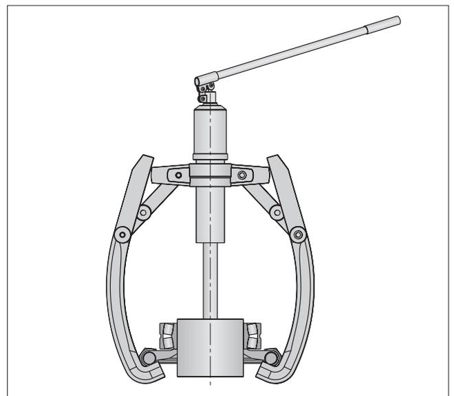
Use of a three-section extraction plate prevents damage because the forces act on the tightly fitted inner rings.
