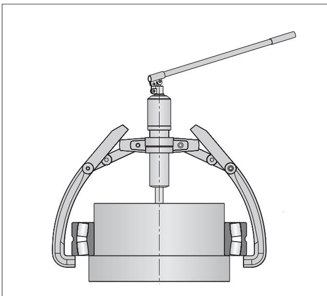
If the extraction forces are directed through the rolling elements, the rolling elements and raceways could be damaged.
