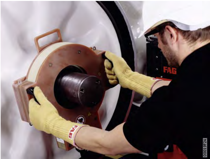
Figure 2 Rigid inductor in the dismounting of wheelset bearings
