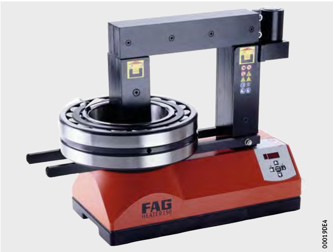
Figure 2 Heating a rolling bearing
