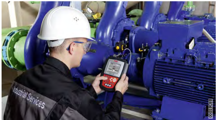
Figure 5 Shaft alignment device FAG Top-Laser EQUILIGN
